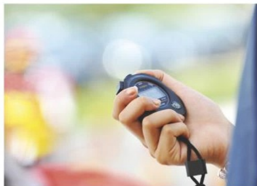
Figure 5 Despite the fact that a stopwatch has a high resolution, it is not always the most appropriate instrument to use for measuring time
