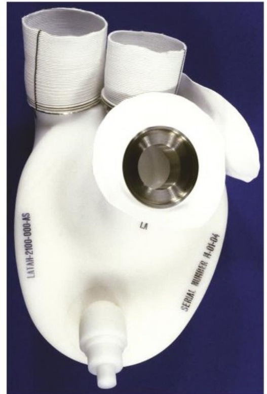
Figure 3 This amazing artificial heart uses air pressure to pump blood around the body
