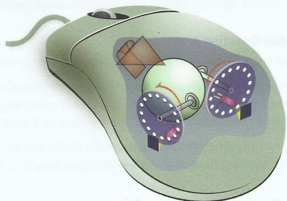
Figure 3.04 The components of a mechanical mouse
