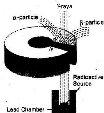
vacuum pumps so that radiation may not absorb air. A permanent magnetic field was applied on this chamber perpendicular to the plane of paper and directed inwards.
