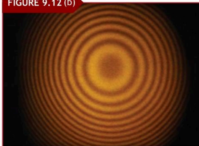
Fringes produced with a Michelson interferometer.
