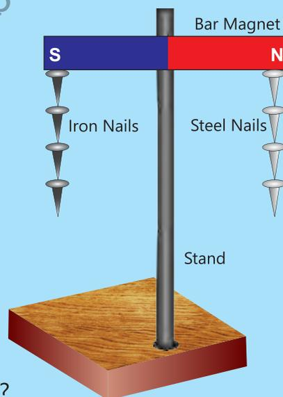
You will see that iron chain collapses whereas the steel chain did not. It means that iron nails temporarily become magnets. On the other hand, steel nails retain their magnetism and become permanent magnets.
