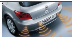
Figure 10.11 (f): Parking sensor system
