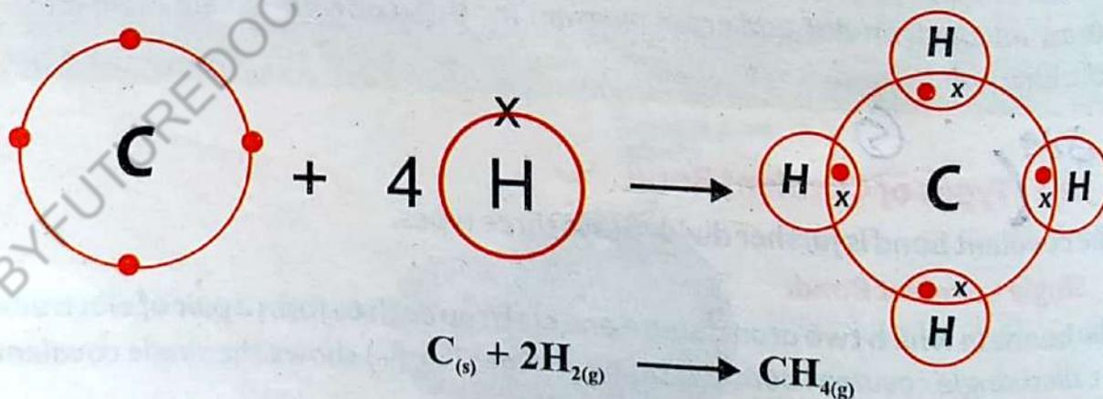
Fig. 4.7 Molecule of Methane
