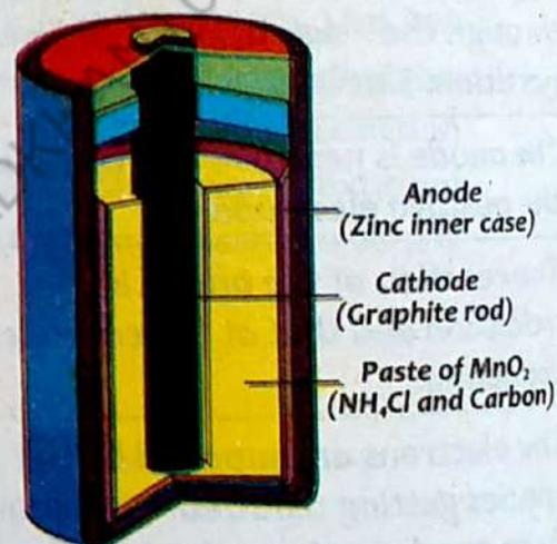
Fig. 7.8 Internal structure of dry cell
