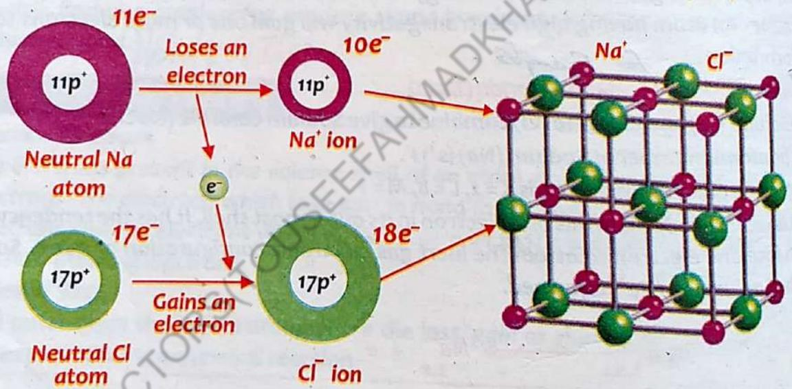
Fig. 4.2 Formation of NaCl compound
