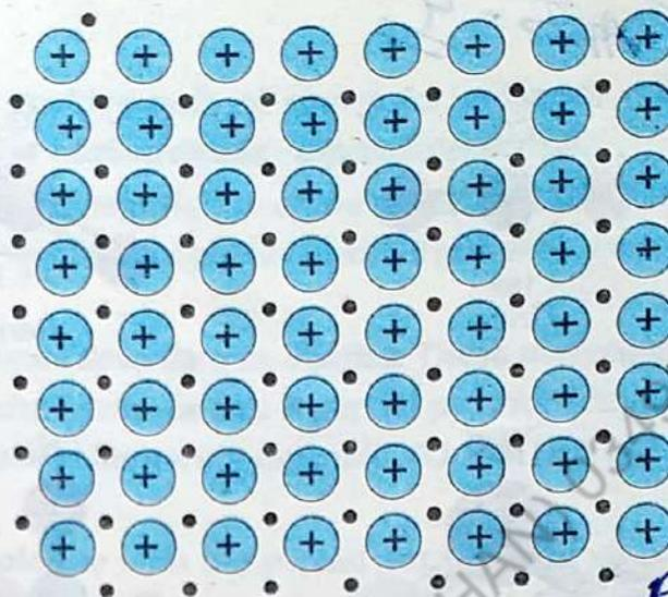
Fig. 4.17 Metallic bonding
