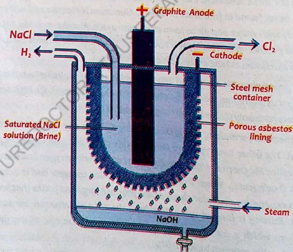
Fig. 7.10 Electrolysis of Aqueous NaCl (Nelson's Cell)
