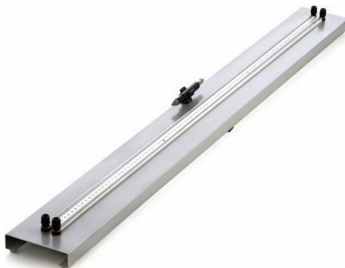
Figure 14.40 A wire potentiometer.
