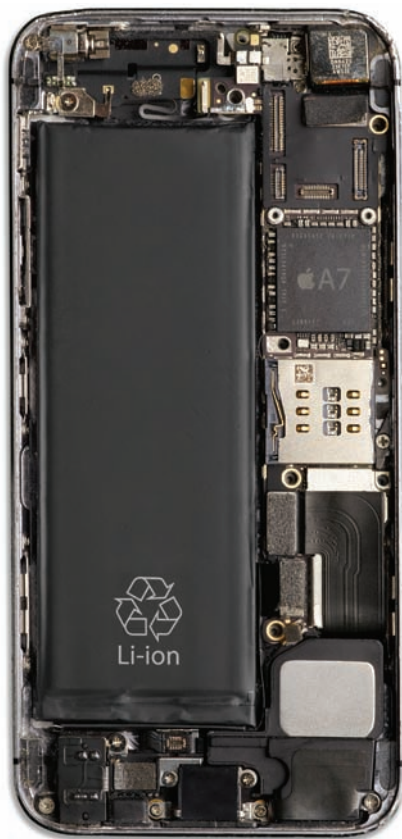
Figure 14.9 The iPhone 5s A7 processor.
