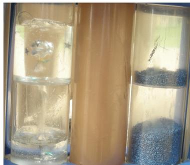
**Fig. -15.12** – Picture of Counter-current flow in liquid–gas and solid–gas configurations. The container is made of two compartments. The upper compartment is filled with the heavy phase (liquid, water solution, or small wood particles) by rotating the container. Even though the solid–gas ratio is smaller, it can be noticed that the solid–gas is faster than the liquid–gas flow.
