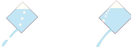
Fig. -15.11 – Counter-current flow in a can (the left figure) has only one hole thus pulse flow and a flow with two holes (right picture).
