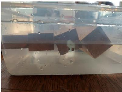
(a) Wooden block floating in a water with a density ratio of around 0.6.
