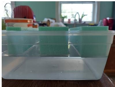
(b) Foam block floating in a water with a density ratio of around 0.05.
