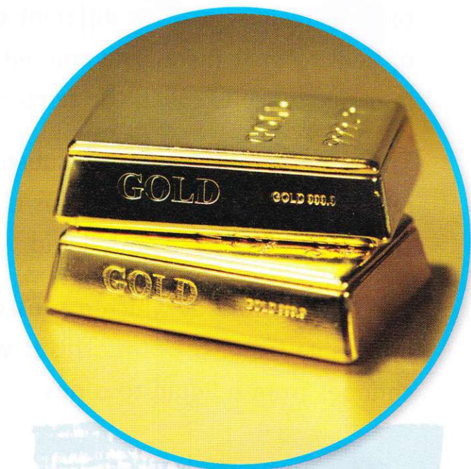
The gold cools in the mould and becomes a solid again. These solid gold bars are called ingots.
