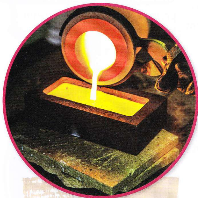
This gold was heated until it melted. Then it was poured into moulds.
