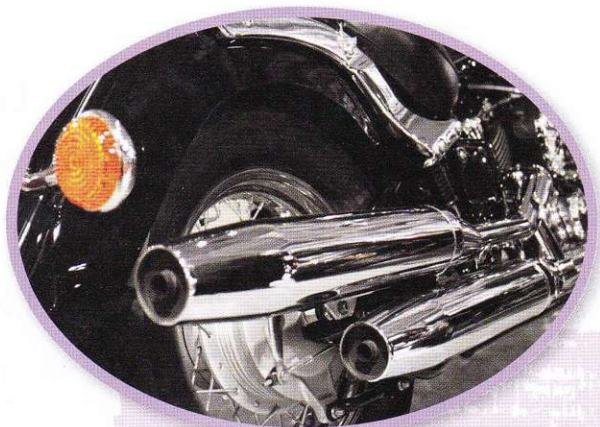
This motorbike silencer muffles the sounds of the engine.
