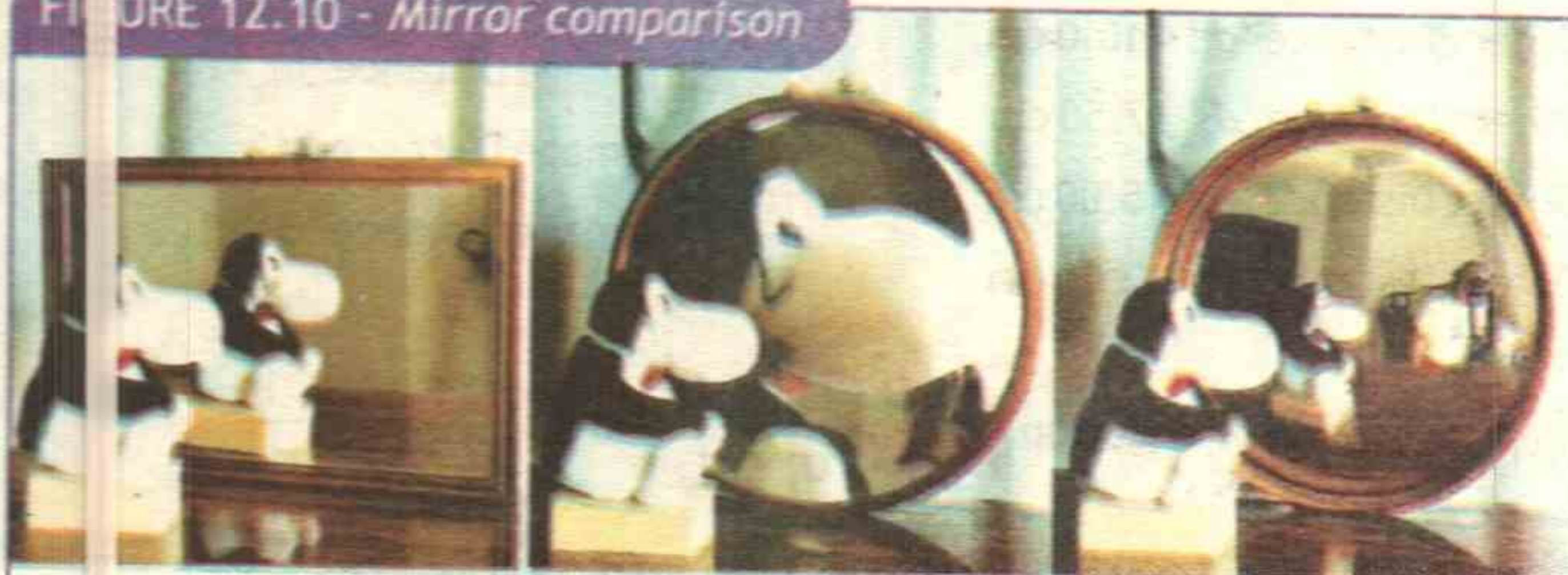
(a) Plane mirror image (no magnification). (b) Enlarged image in a concave mirror. (c) Reduced image in a convex mirror.
