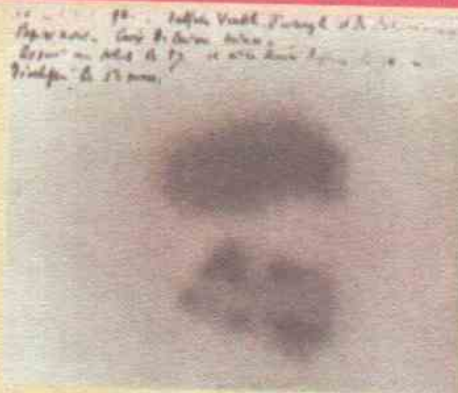
Becquerel's photographic plate. The bottom of the image shows shadow cast due to absorbed radiation.
