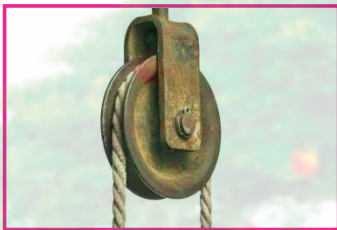
Rope and Pulley are used to draw water from the well.
