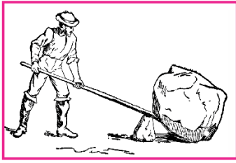
Lever is used to lift heavy load.
