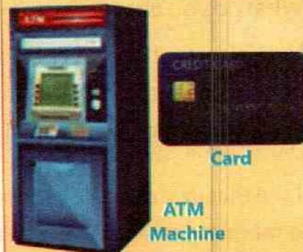
A magnetic chip is built in a credit card of a bank. The ATM machine is programmed to read the data of the user present in the chip.
