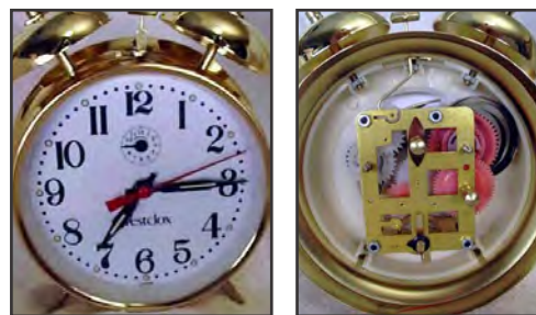
Fig.9.17: Gear system in a wind-up clock
